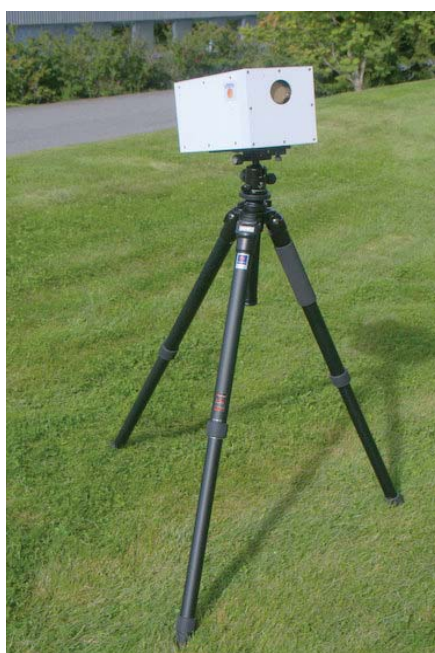
Left-panels. Temperature image of a thermal power plant plume in Iceland and the corresponding temperature histogram (bottom left). Centre panel. NicAIR mounted on tripod. Right panels. Filtered infrared temperature images (top four panels); derived \text{SO}_2 image (bottom left) and corresponding digital camera photograph of Turrialba, Costa Rica, volcanic emissions.
