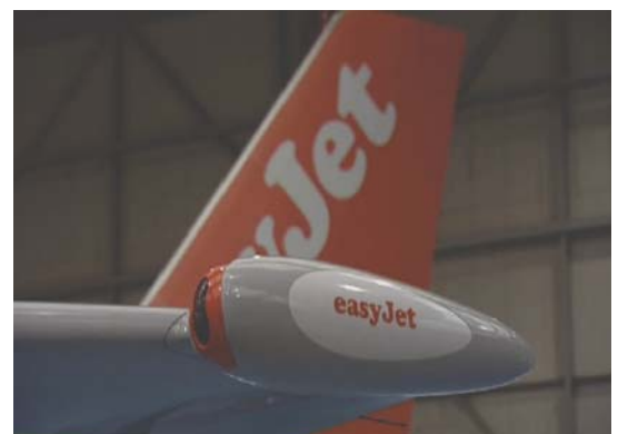
Figure 2. The AVOID system mounted at the wing-tip of an easyJet A320.
